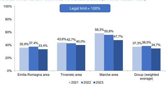
The indicator relates to plants with more than ten thousand population equivalent (the volumes treated in these plants are 93% of the total effluent treated) and is calculated on the basis of the ratio between the measured concentration of Bod5, Cod, Sst, ammoniacal nitrogen, phosphorus and total nitrogen and the relevant maximum concentrations permitted by Legislative Decree. 152/2006 or by the authorisations in force for the individual plants.
